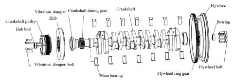
Figure 41 Exploded view of crankshaft group
