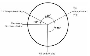
Figure 40 Schematic diagram for included angles between piston rings
