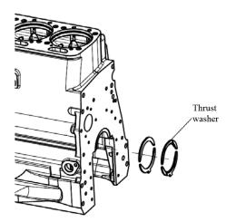
Figure 34 Exploded view of thrust washer
