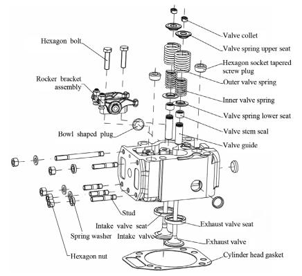
Figure 20 Exploded view of cylinder head assembly
