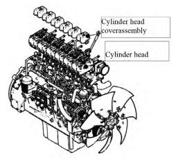
Figure 18 Exploded View of Cylinder Head Group
