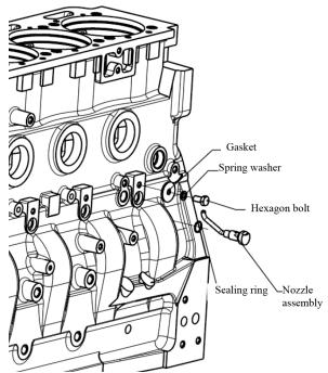
Figure 33 Exploded view of piston cooling nozzle
