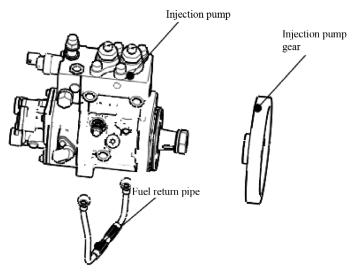
Figure 59 Exploded view of injection pump
