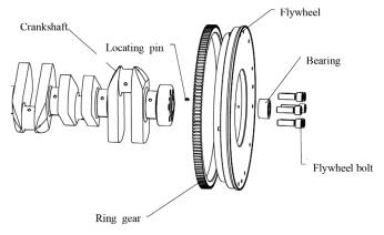
Figure 43 Exploded view of flywheel and ring gear
