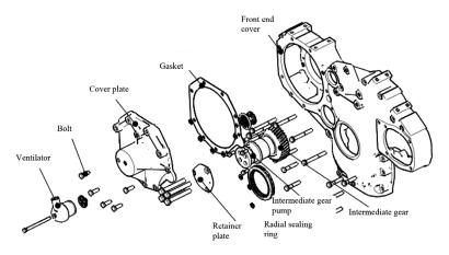
Figure 28 Exploded view of front end cover
