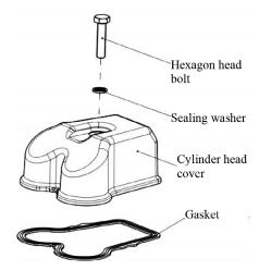
Figure 19 Exploded View of Cylinder Head Cover Assembly
