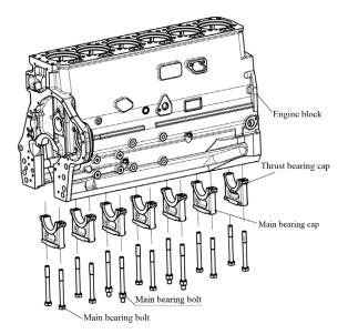
Figure 26 Exploded view of engine block assembly
