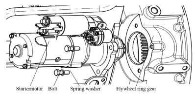
Figure 67 Exploded view of starting system
