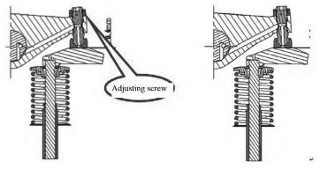
Figure 14 Adjusting screw
