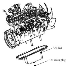
Figure 32 Exploded view of oil pan
