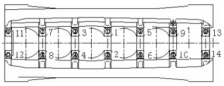
Figure 27 Tighteningsequencefor main bearing bolts
