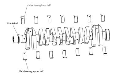
Figure 45 Exploded view of crankshaft bearing
