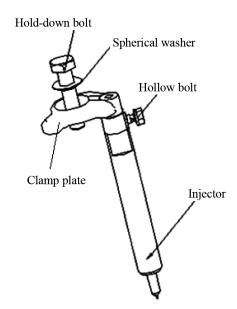
Figure 61 Exploded view of injector
