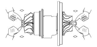
Figure 57 Measuring of radialplay
