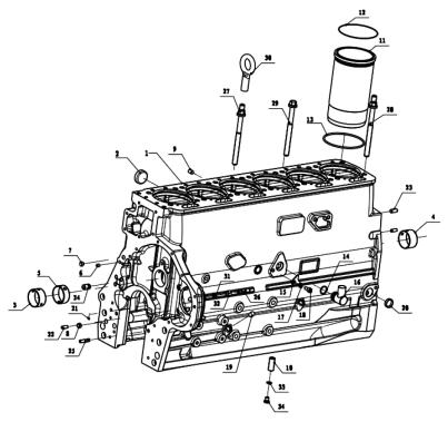
1-Engine block; 2, 20-Bowl shaped plug; 3, 4, 5-Camshaft bush; 6, 7, 8, 9-Plug; 11-Cylinder liner; 12, 13, 14-O-ring; 15-Retaining plate; 16-Welded elbow; 17, 31-Spring washer; 18-Hexagon socket cap screw; 19, 22, 23-Straight pin; 21-Spring-type straight pin; 24-Pin shaft; 25, 26-Stud; 27, 28, 29-Cylinder head bolt; 30-Eye ring screw; 32-Hexagon nut (Type 2); 34-Hexagon screw plug
