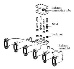
Figure 54 Exploded view of exhaust manifold
