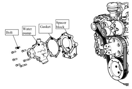
Figure 65 Exploded view of water pump assembly
