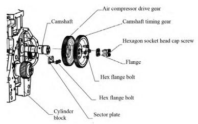
Figure 47 Exploded view of camshaft
