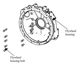
Figure 30 Exploded view of flywheel housing
