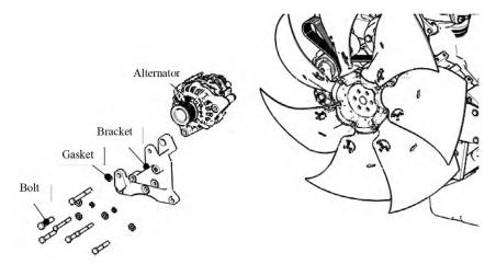
Figure 68 Exploded view of accessories
