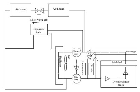
Figure 63 Cooling system loop of WP6 series diesel engine
