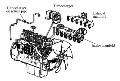
Figure 52 Exploded view of intake/exhaust system
