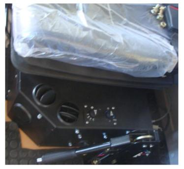
The heater and air conditioner are combined into one blower unit under the operator's seat. If necessary, the operator can control inner temperature using the operation panel installed in the top of the evaporator;
