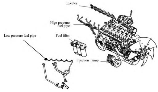
Figure 58 Exploded view of fuel system
