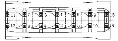
Figure 42 Tightening sequence for main bearing bolts
