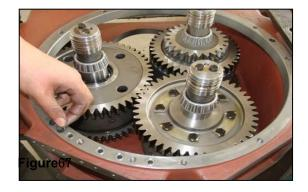
10. Install reverse gear bearing sleeve and reverse gear clutch.
