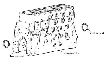
Figure 35 Exploded view of front/rear oil seals
