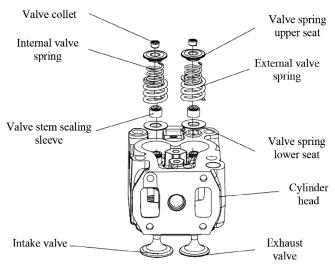
Figure 50 Exploded view of valve
