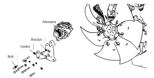
Figure 69 Exploded view of alternator
