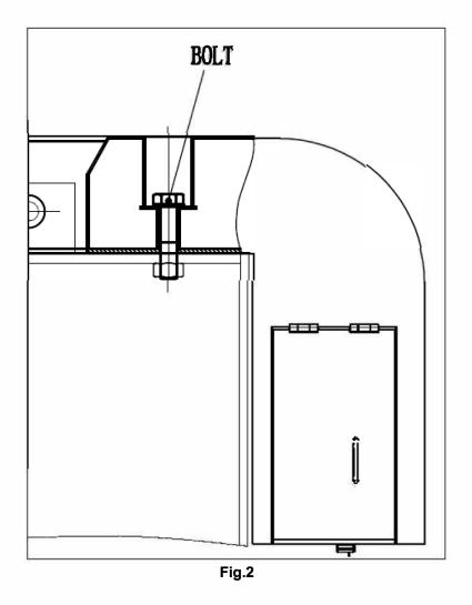
**NOTE: 1**) Tighten bolt to torque value list in the following table.
