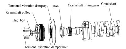
Figure 44 Exploded view of torsional vibration damper, pulley and hub
