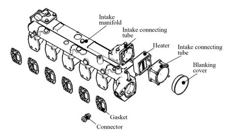
Figure 53 Exploded view of intake manifold
