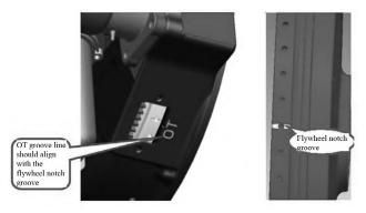
Figure 12 Flywheel notch groove
