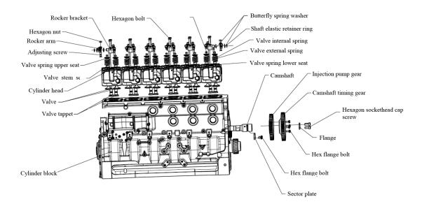
Figure 46 Exploded view of valve train
