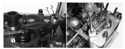
Figure 13 Adjustment of valve clearance
