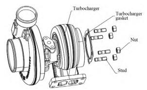
Figure 55 Exploded view of turbocharger system
