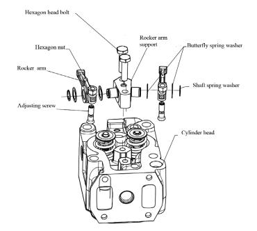
Figure 48 Exploded view of rocker arm and rocker shaft
