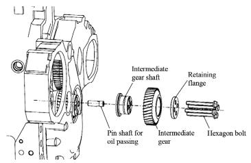
Figure 51 Exploded view of intermediate gear
