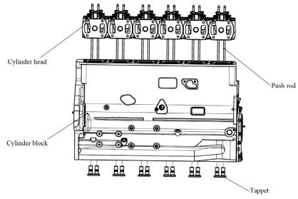
Figure 49 Exploded view of tappet and push rod
