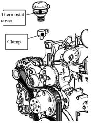
Figure 66 Exploded view of thermostat assembly
