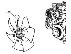
Figure 64 Exploded view of fan assembly
