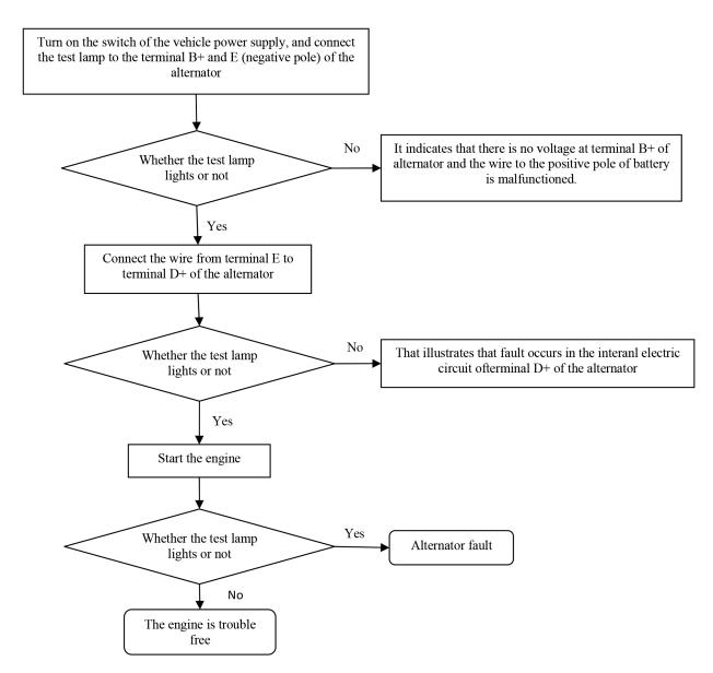
Figure 70 Diagnosis Trouble Flow Chart for Alternator
